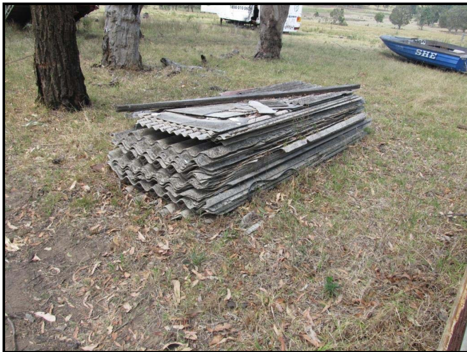
Photo 8: Photograph of a stockpile of asbestos roof sheeting located north of the dwelling.
